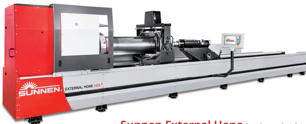
**Sunnen External Hone** has been developed to meet the continuously increasing demands of the industry. Workpieces in the offshore, energy production and aviation sectors are exposed to extreme environments. Therefore electroplated hardchrome or plasma-spray coated surfaces are in operation. The new HES machine cuts nearly all advanced materials without trouble.
