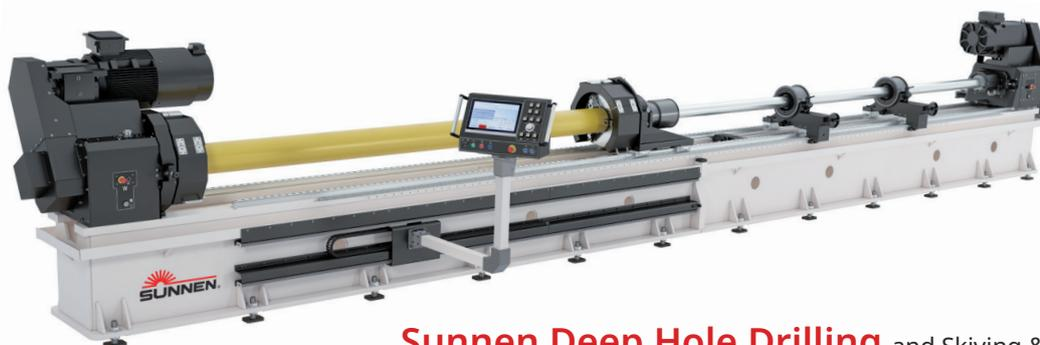
**Sunnen Deep Hole Drilling** and Skiving & Roller burnishing systems are cost effective bore sizing solutions for hydraulic cylinders and other high production applications. Sunnen is unique in offering single-source turnkey solutions for your deep hole drilling and skiving and roller burnishing applications, including machines, tools, inserts, cutting oils and filtration units.
