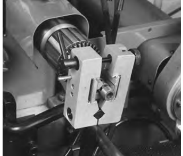
FB-E External Hone Body with MB-750 External Adapter Chuck in MBB-1660 Horizontal Hone.
